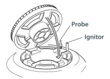
Fig. 20 Fitting the burner spreader to the housing.
